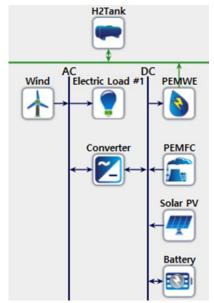
Figure 5: HOMER simulation model
