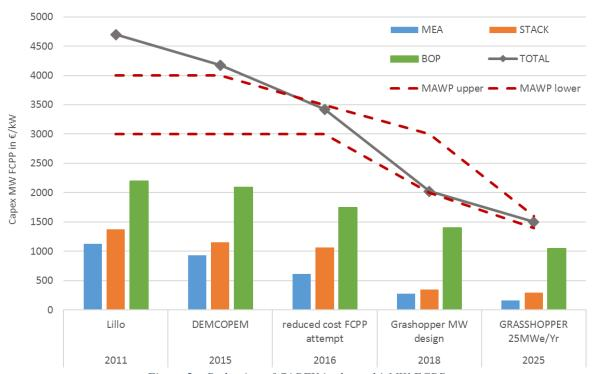
Figure 2 – Reduction of CAPEX in the multi-MW FCPP.
