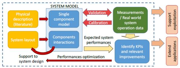
Figure 5 - Conceptual scheme of general modelling activities connected with field measurement and their impact on system performances optimization
