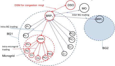
Fig.4: Schematic representation of Use case 2 with players, roles, processes and relations [4].
